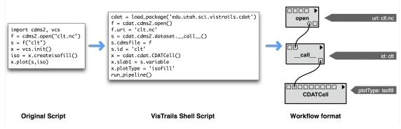
Figure 38: Simple UV-CDAT Python script opening a file and plotting a 2 dimensional contour plot
